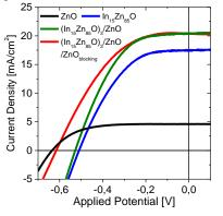
Figure 2. *J-V curves* of the devices featuring different photoanodes
